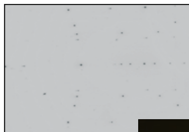
colloidal goethite nanorods 50 \mu beam size, bending magnet BM26 @ ESRF
