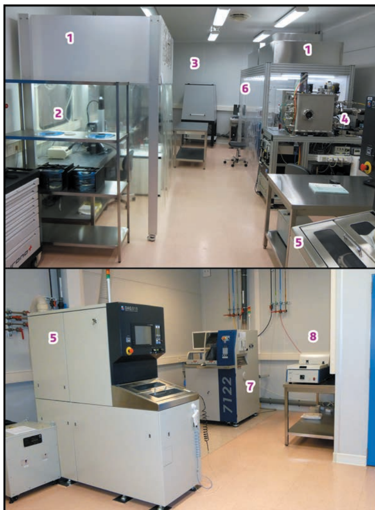
Fig. 152: View of the CAL “clean room” with main processing tools. 1) Laminar flow hoods; 2) 3-axis-robot with glue dispenser; 3) Micro-interferometer; 4) Semi-automatic anodic bonding machine; 5) Grinding machine; 6) Spin coater; 7) wafer dicing saw; 8) wafer mounting machine.
