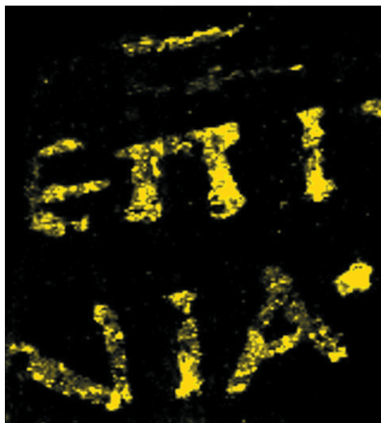
Fig. 36: X-ray fluorescence micro-imaging technique reveals the lead contained in the ink.
