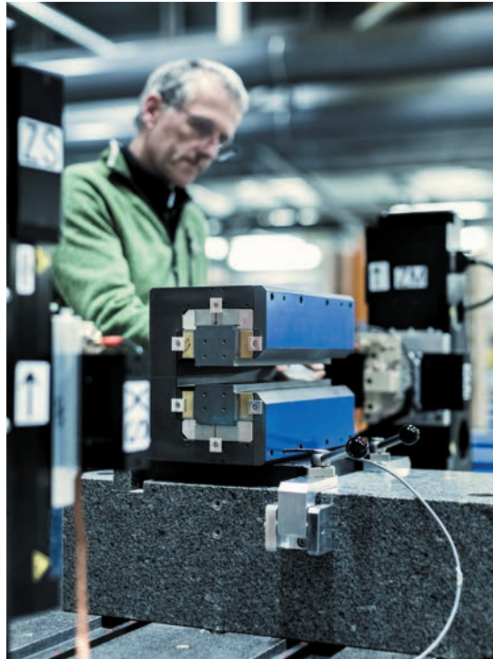
Fig. 3: Joel Chavanne takes magnetic measurements of one of the dipole magnet modules.
